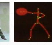
Kinect®: motion sensing input device for Xbox and Windows; Comprise an infra-red and a RGB webcam; Detect coordinates of the human skeleton
